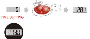
Press the "MODE" button for a few seconds to turn on the time setting function.
